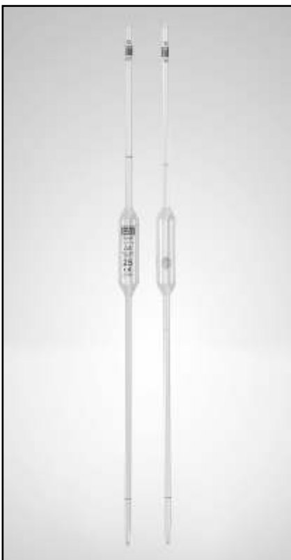
Volumetric pipette, class 'AS' EM-Techcolor
