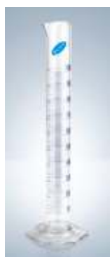
Cylinders, Measuring, Class 'A', Graduated, with Individual Certificate of Performance, Made from Heat Resistant, Low Expansion Borosilicate Glass, RIVIERA
